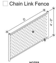
50mm (2") spacing (B), if rail spacing is < 3'-0" (A) 38mm (1.5") spacing (B), if rail spacing is > 3'-0" (A)
