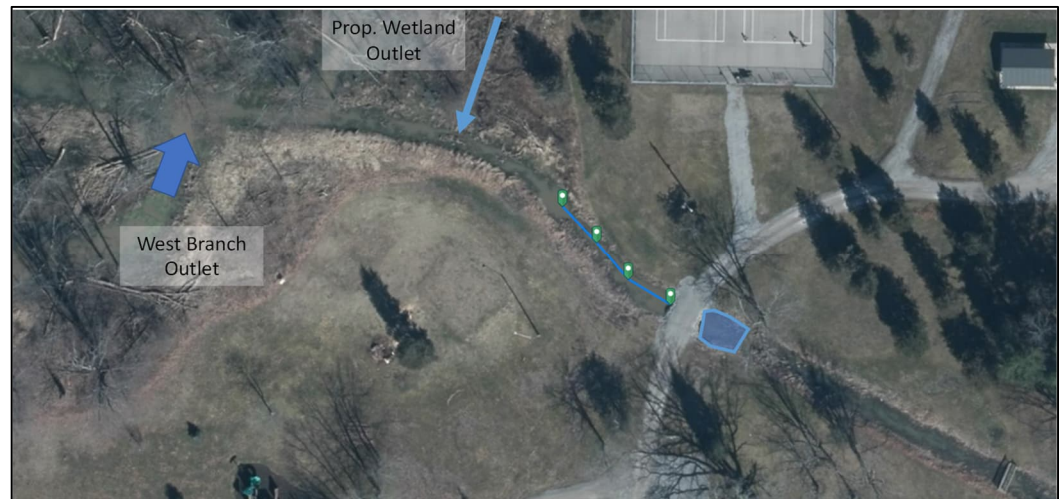
Figure 9 Centennial Park Culverts Proposed Riffles and Pool
