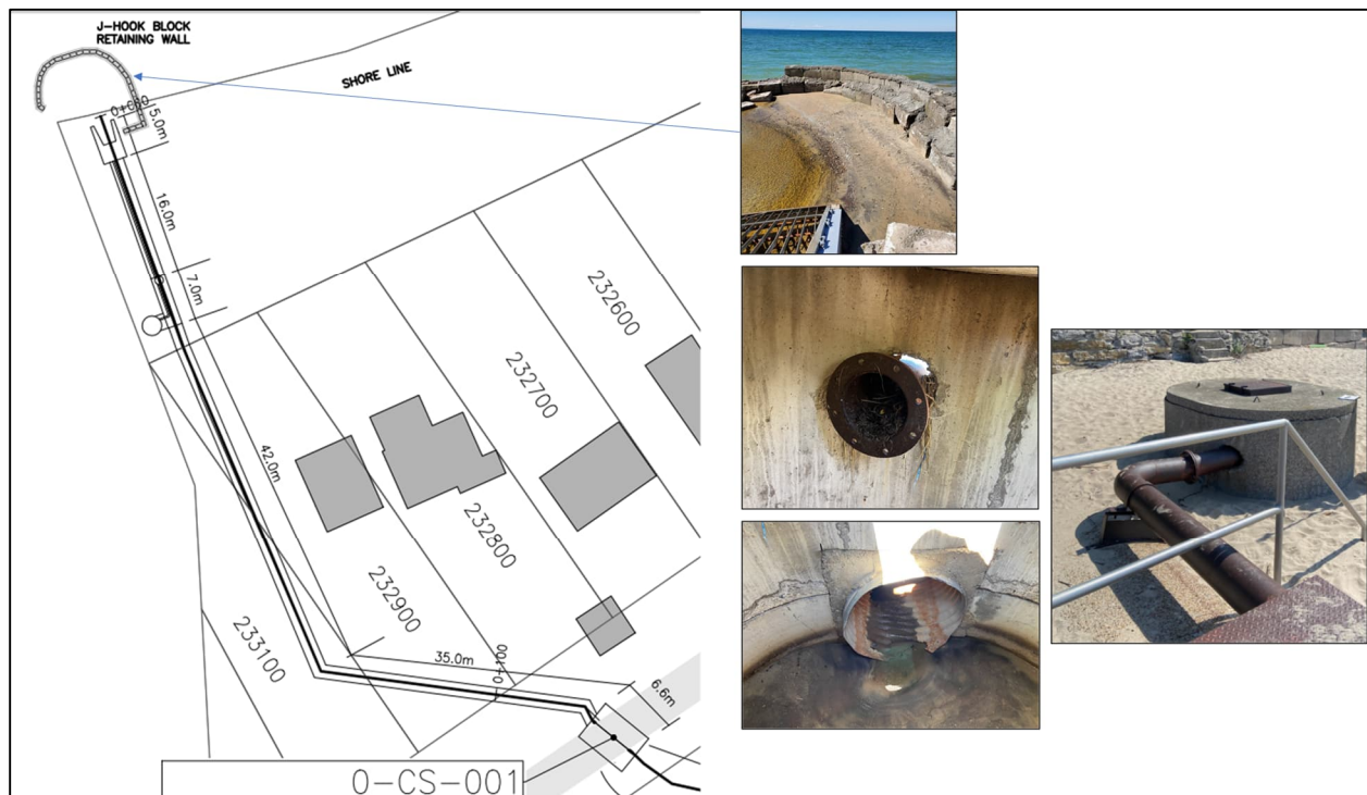
Figure 26 Oil Mill Creek Control Structure and Pump
