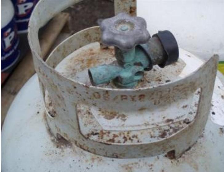
Also, if you have a 20-pound propane cylinder with a valve that is green in colour, do not use the cylinder and return it to the supplier.
