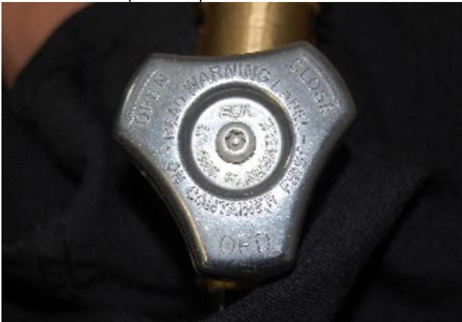
The safety issue involves cylinders that have been sent to retail cylinder exchange facilities that may have their cylinder valve left in the open position. Connection of the supply hose to the propane cylinder when the valve is in the open position could result in the release of propane creating the risk of fire. The OFM and the Technical Standards and Safety Authority (TSSA) are urging anyone who has purchased a 20-pound propane cylinder that is identified with a label
