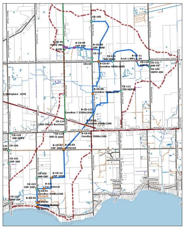
Figure 22 Beaver Dam Bridge and Culvert Drain Structures
