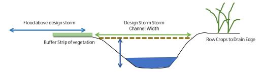
Figure 11 Cross-section ditch view
