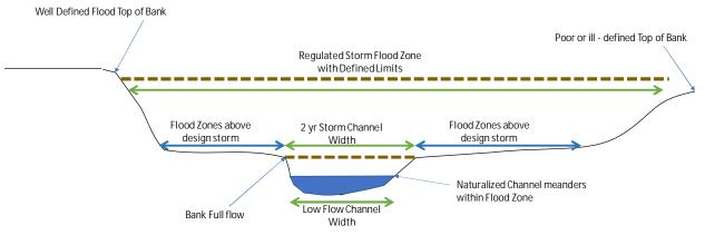
Figure 13 Naturalized Channel cross-section
