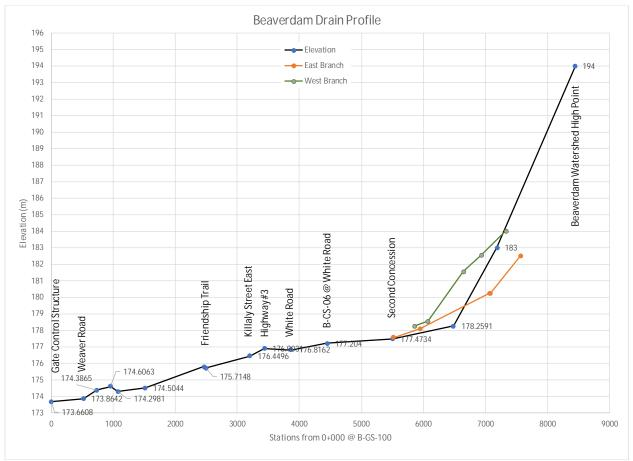
Figure 16 Beaver Dam Drain Profile
