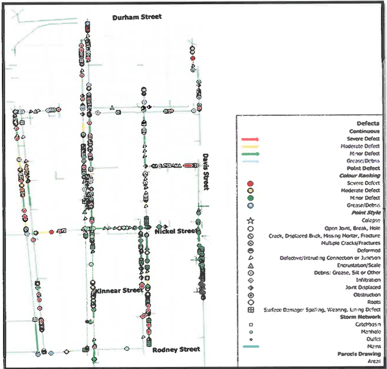
Figure 2-6 Nickel Area Storm Sewer Inspection Observations
